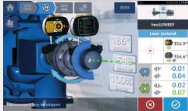
As shafts are rotated, measurement quality is clearly displayed – a green or blue sector indicates good measurement data.
